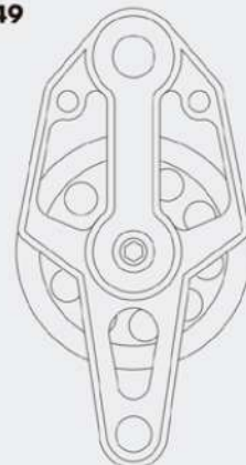
Simples fixo/saida para runner Single fixed head/becket for runner
