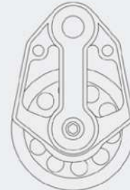
Simples fixo para runner Single fixed head for runner
