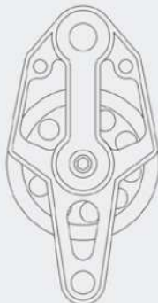
Simples fixo/saida para runner Single fixed head/becket for runner
