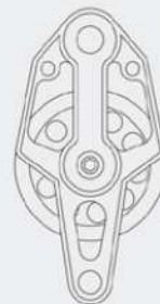
Simples fixo/saida para runner Single fixed head/becket for runner
